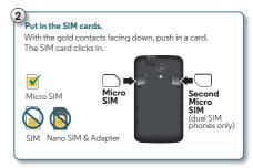
Note: To remove a SIM card, push it in to release it. Then slide it out.
